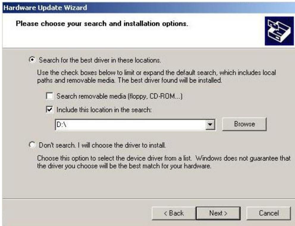
From here you will click *Browse* to navigate the driver installer to the path where the drivers are located, either on your CD or on your hard drive. Choose the appropriate folder based on the DVR Card (HC1, HC2, HC3), the operating system, and the architecture (32-bit or 64-bit). For example if you purchased a HC2 Platinum card and you are using Windows XP 32-bit, then you would select:
